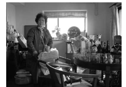
Figure 6. This photograph shows interior damage on the 9th floor of a 16 story condominium; because damage to the lower stories produced a seismic isolation effect, shaking in the upper floors was amplified and home contents were scattered.
