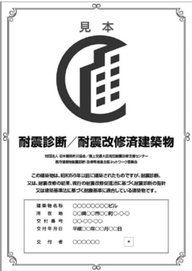
Figure 1. After the completion of strengthening works, an inspection plaque acting as a “mark of conformity” may be displayed to confirm the building meets earthquake resistance standards (by the Japan Building Disaster Prevention Association).
